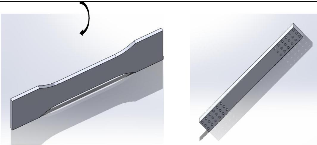
**Figure 1:** Tensile and Flexural Specimens: (a) ASTM D638 tensile dimensions, (b) ASTM D790 flexural dimensions, (c) 3D tensile model, (d) 3D flexural model.
