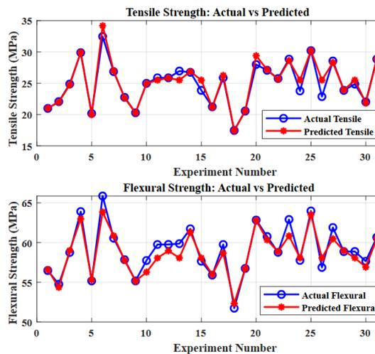
**Figure 6** Comparison of Actual vs Predicted Tensile and Flexural Strengths
