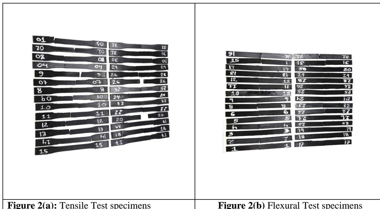
Figure 2(a): Tensile Test specimens
