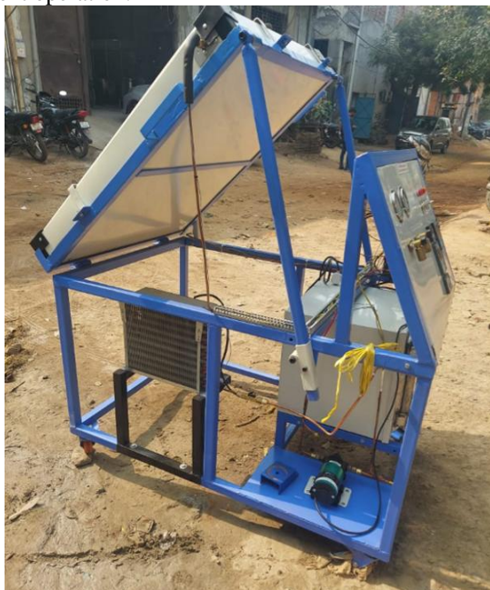
Figure 8. Final Fabrication of Solar Thermal Adsorption Refrigeration System
