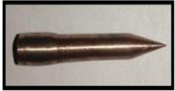
Figure 3: Cu Tool Electrode (Tip Dia- 0.15mm)
