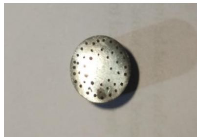
Figure 9: Textured Pin (Workpiece)
