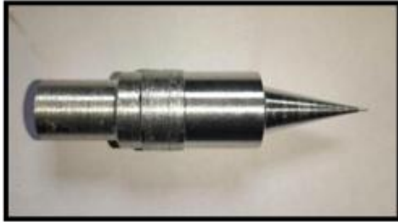
Figure 2: Al tool electrode (Tip Dia.- 0.5mm)
